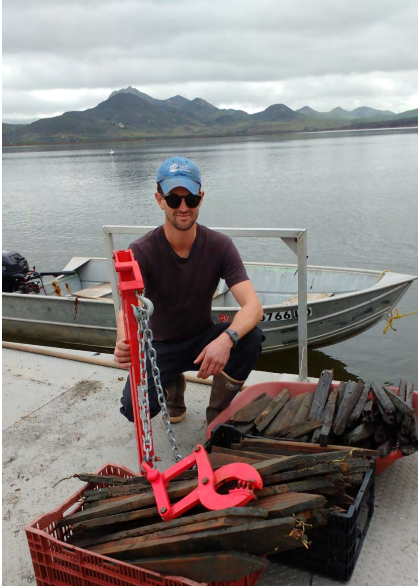
Figure 6. Farm Manager Charles Trevelyan with the tool he developed for extracting posts. The jaw like part is a pallet puller which is chained to a post puller. On this day the tool was used to remove wooden stakes. The stakes in the front 2 bins are made of 1"x4" untreated lumber and were previously used by GBOC to support racks. We removed them because they rotted too quickly. The stakes in the rear-most bin are mostly old "legacy" stakes from a previous grower.
